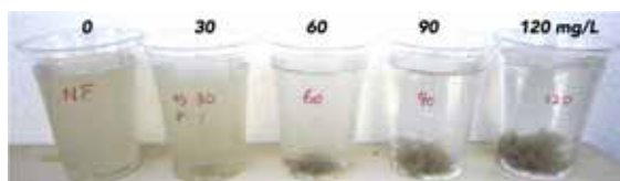
図 - 12 PFPW Trial Jar Tests: 2 nd AS addition
