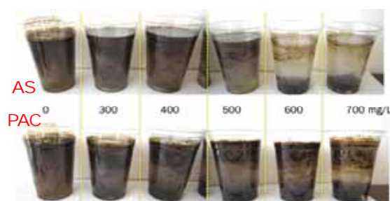
図 - 10 PFPW Trial Jar Tests: AS vs. PAC addition
