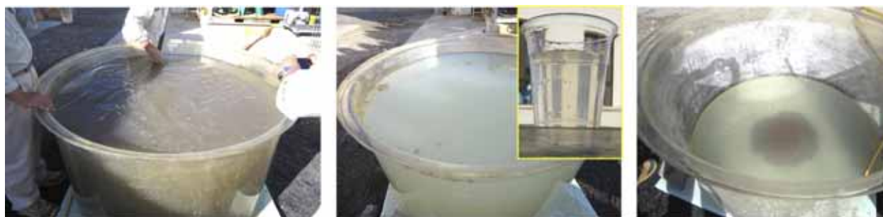
図 - 13 PFPW Trial Jar Tests: 2 nd AS addition for 1m 3 Tank. Test
